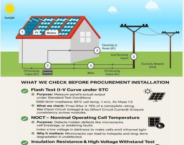
Purpose: Ensure the panel can safely handle high voltages without breakdown
